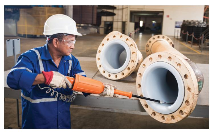
programme to obtain uniform lining thickness throughout internal surface of fittings within tolerance limit. Precise process control ensures seamless continuous smooth finished internal lining even at edges, corners and welded beads.
